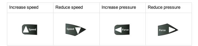
The cutting speed and contact pressure cannot be changed while a plotting job is in progress.
